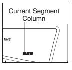
will be shown in the flashing Current Segment column of the matrix. (The incline settings are not shown in the matrix.) To program a speed setting and an incline setting for the first segment, simply adjust the speed and incline of the treadmill as desired by pressing the Speed and Incline buttons. Every few times one of the Speed buttons is pressed, an additional indicator will appear or disappear in the Current Segment column.
